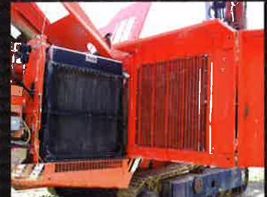
Drilling Rig Air Intake
